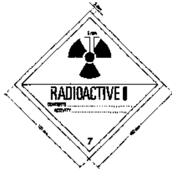
Fig. 2. Category I-WHITE label. The background colour of the label shall be white, the colour of the trefoil and the printing shall be black, and the colour of the category bar shall be red.
