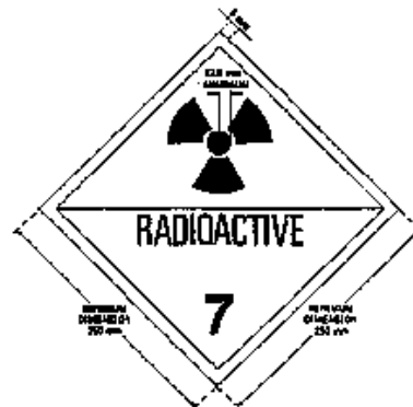
Fig. 5. Placard. Minimum dimensions are given: when larger dimensions are used the relative proportions must be maintained. The figure "7" shall not be less than 25 mm high. The background colour of the upper half of the placard shall be yellow and the lower half white, the colour of the trefoil and the printing shall be black. The use of the word "RADIOACTIVE" in the bottom half is optional to allow the alternative use of this placard to display the appropriate United Nations Number for the consignment.
